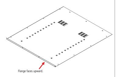
**3.** Attach the left side (Ref. No. 2) to the back by placing flange (A) around the back and bolting the back and side together with four bolts and nuts (Ref. Nos. 15 & 16). Be sure that the lances on all shelf adjustment strips (B) point in the same direction.
