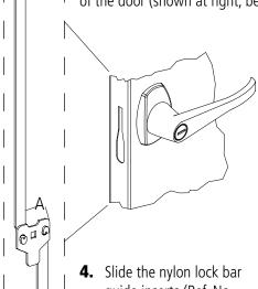
**4.** Slide the nylon lock bar guide inserts (Ref. No. 11) over the lock bar ends and through the door slots (see "B" at right). Push down firmly until the guides snap into place.
