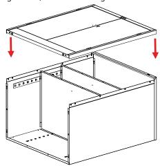
**7.** Set the unit upright and attach the top (Ref. No. 5) by inserting the weld-studs into the holes provided on the left and right sides. The flange should fit over the outside of the rear of the cabinet, and theoffset should be toward the front. Bolt together by attaching nuts to the weld studs and inserting bolts and nuts through the holes along the back edge.
