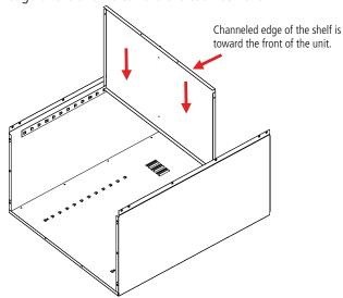
**6.** Place the second shelf at the desired level in the same manner as in step 5. Next, attach the door frame assembly (Ref. No. 6) to the cabinet body by placing it over the sides. Align the weld studs with the slots in the left and right sides, and attach using four nuts on each side.
