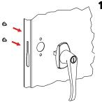
1. Place the locking handle (Ref. No. 9) on the right hand door and fasten with two #8-32 X 1/4 hex-head bolts and lock washers, provided with the handle.
