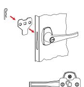
With the handle still in the open position, hook the locking bars (Ref. No. 8) to the locking cam (see "A" at left). Once in position, slowly rotate the door handle to the closed position so the lock bars prot rude from the holes at the top and bottom of the door (shown at right, below).
