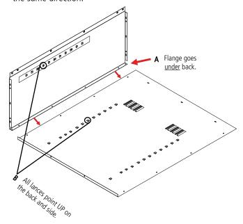
**4.** Attach the right side (Ref. No. 3) to the back in the same manner as in step 3, again making sure that the flange is around the back and that
